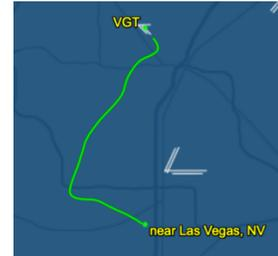
**Meanwhile** he appeared to maintain control, flying an approximately steady groundspeed that, with surface winds from the south, is consistent with flight at or near  $V_{YSE}$  (“blue line”) speed...what you’re supposed to do on one engine close to the ground. Altitude was apparently controlled as well, more or less level before a gradual descent.
