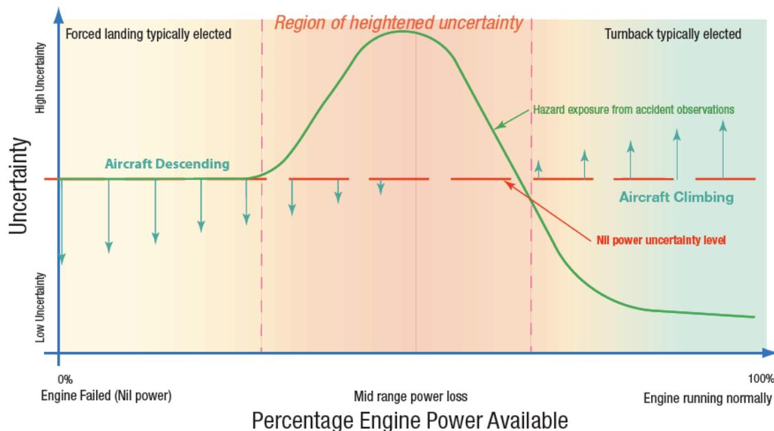
**ATSB’s research** shows that a slight power loss after takeoff (toward the right of the ATSB chart above) may not be enough to prevent a safe return to the aerodrome, er, airport, for a (fairly) normal landing. Conversely, a nearly total engine failure (toward the left of the chart) gives the pilot little choice to descend, and at least in Australia’s recent history the pilot usually continued straight ahead...and survived.
